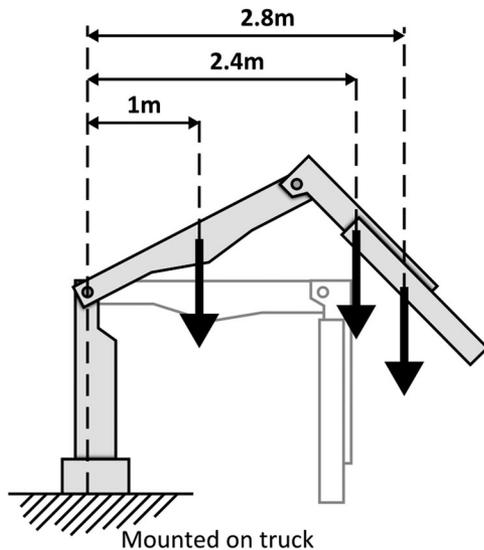
**Figure 2** Scheme of the truck-mounted crane, the different parts, and how moment allocation has been performed. m = meters.
