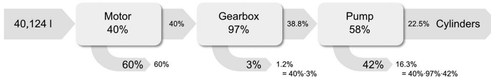
**Figure 3** Scheme of the losses and consumption in different components outside of the crane. l = liters.
