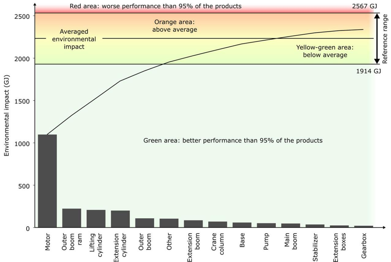
**Figure 4** Pareto graph of the new crane including reference ranges (x-axis: crane components; y-axis: environmental impact using cumulative energy demand as indicator). GJ = gigajoules.
